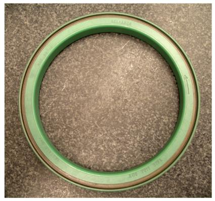
The current replacement crankshaft seals for the John Deere 300 and 350 series engines utilize an integrated wear sleeve and are called "unitized" or "cassette" type seals. These seals will be rendered unusable if they have been separated from their wear sleeves and should be discarded and replaced if this occurs. The appropriate installer tool (JDE30040 or equivalent) MUST be used to ensure proper seal installation.
