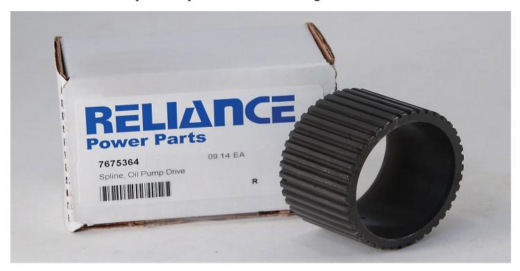
Reliance Parts Corporation is pleased to announce the availability of replacement oil pump drive splines for International D312, D360, D/DT414, D/DT436, and DT466 engines. The drive spline in these applications is installed in front of the crankshaft gear and must be replaced any time the crankshaft gear is replaced.
